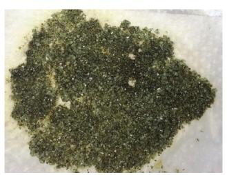
Figure 4 - Fine sand recovered during swabbing operations (1st June, 2014)
