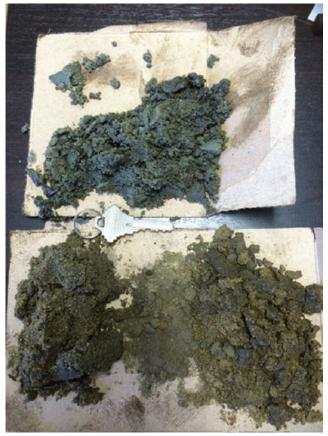
Figure 3 - Fine sand and clay recovered during swabbing operations (1st June, 2014)
