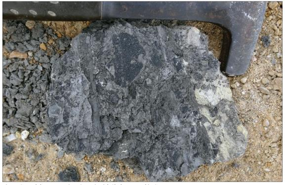
Figure 6 – Malubog Formation: Organic Rich Shale Exposed in Quarry
