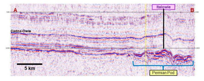
Figure 4: Italowie Exploration Lead – Seismic Section
