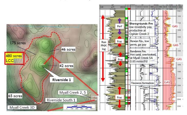
The Riverside Gas Field was later covered by a 3D seismic survey and mapping of these data led to an interpreted 480 acres of closure – a reasonable sized structure. GGX will fund the drilling of one well to basement which will be located on the northern structural high. This well is considered as an appraisal well for gas production.
