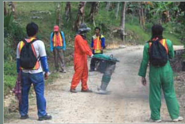
Figure 6 - SC 44: Mini-Sosie Seismic Survey in process
